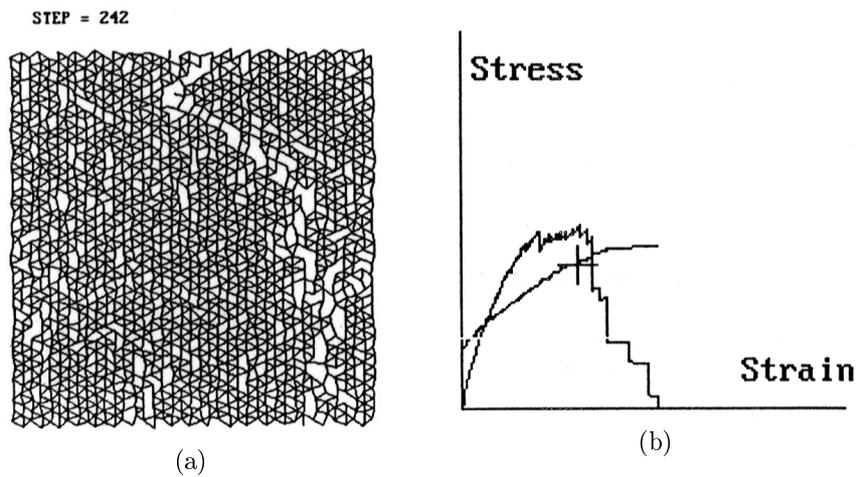
Figure 3: The final failure state (a) and the corresponding load - displacement (the upper one) and damage - displacement (the lower one) curves (b). The cross (+) indicates the alarm for the coming damage localization.
