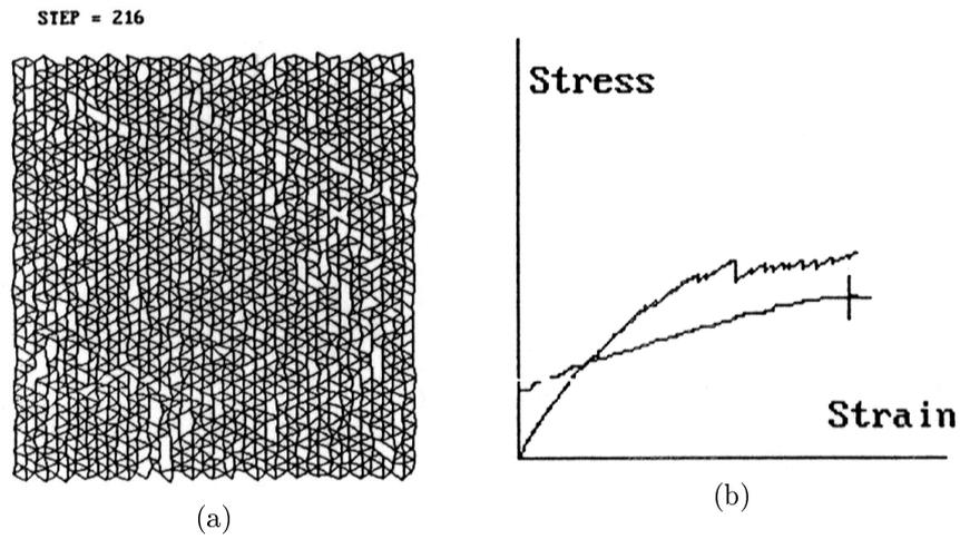
Figure 2: The microdamage pattern at the moment when the criterion for damage localization (6) gives alarm (a) and the corresponding load - displacement (the upper one) and damage - displacement (the lower one) curves (b). The cross (+) indicates the alarm for the coming damage localization.
