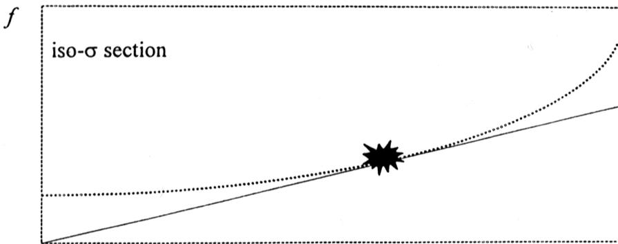
Figure 1: Schematic lower bound for damage localization  $f_d \geq f/D$
