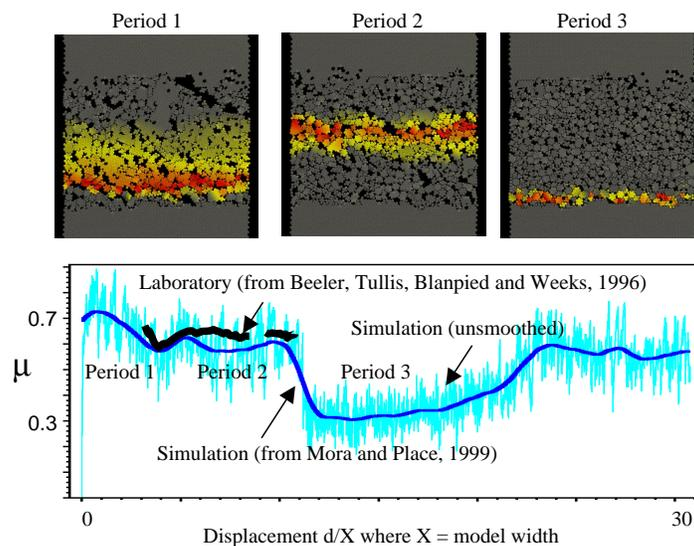
Figure 3: **Top:** Snapshots showing how shear strain in a fault gouge layer localizes into a narrow band. The lighter grey depicts the zone of active shear. **Bottom:** Fault friction in the numerical experiment compared to that of a long displacement laboratory experiment (note: the horizontal scale of the laboratory derived curve is not the same as the simulation result).
