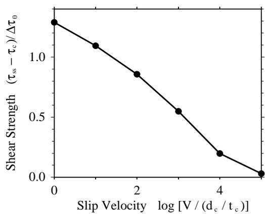
Theoretical slip-velocity dependence of shear strength in steady-state slip. The slip velocity  $V$  is normalized by  $d_c/t_c$ .
