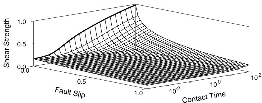
Figure 2: Evolution of constitutive relation after the arrest of a high-speed fault slip. The shear strength  $\tau$ , the fault slip  $w$ , and the contact time  $t$  are normalized by  $\tau_0$ ,  $d_c$ , and  $t_c$ , respectively.
