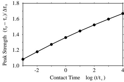
Change in peak strength with time in stationary contact. The contact time  $t$  is normalized by the characteristic healing time  $t_c = (\beta k_c^2)^{-1}$ . The other parameters are the same as in Fig..
