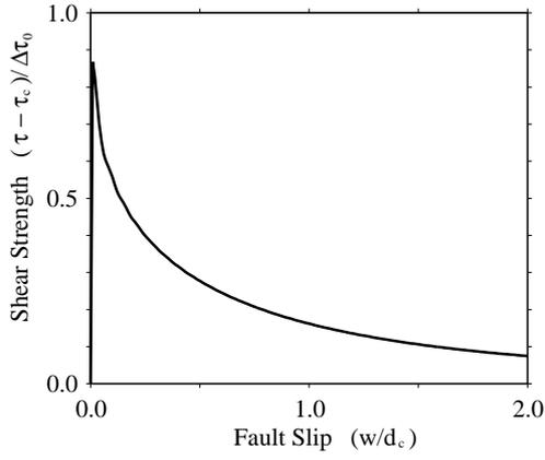
Change in shear strength with fault slip in high-speed slip. The initial values of  $k_c$  (upper fractal limit) and  $k_0$  (lower fractal limit) are taken to be 10 and  $10^4$ , respectively. The strength  $\tau$  is normalized by the initial strength rise  $\Delta\tau_0$  defined by equation (6), and the fault slip  $w$  by the characteristic weakening displacement  $d_c \equiv (\alpha k_c)^{-1}$ .
