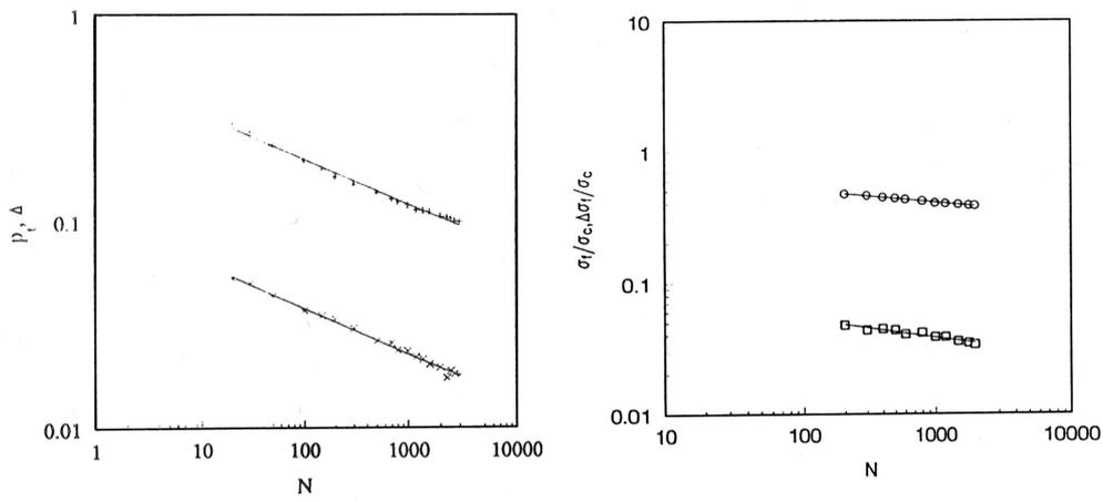
Figure 2: Size effect of transitional region (a)  $p_t$  and  $\Delta$ ,  $\sigma_0/\sigma_c = 0.5$ , + :  $\bar{p}_t$ , x :  $\Delta$ , (b)  $\bar{\sigma}_f$  and  $\Delta\sigma_f$ ,  $p_0 = 0.2$ , o :  $\bar{\sigma}_f/\sigma_c$ , □ :  $\sigma_f/\sigma_c$
