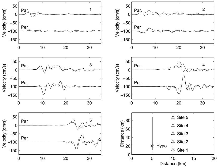
Figure 4: Comparison of synthetics for a kinematic simulation (solid traces) of the Landers earthquake to those for a dynamic simulation (dashed traces) using  $T_u = 80$  bars and  $D_0 = 2$  m. 'Par' and 'Per' depict fault-parallel and fault-perpendicular traces, respectively.
