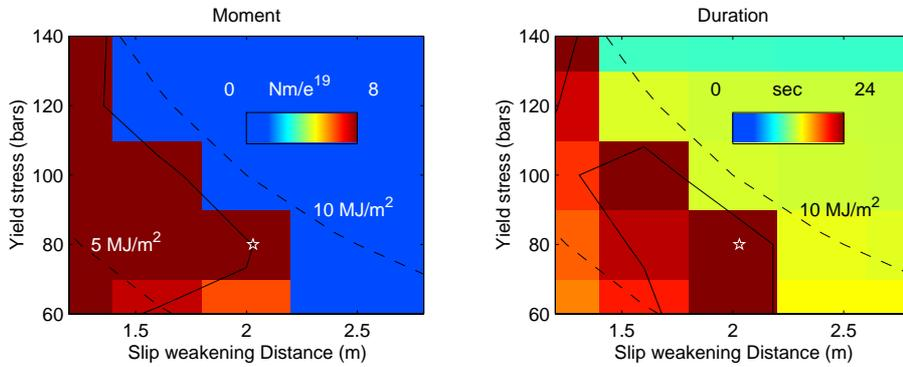
Figure 1: Moment and duration as a function of yield stress and slip weakening. Tectonic stress was 40 bars. The solid contour lines depict values of  $7.7e^{19}$  Nm for the moment, and 24 seconds for the duration plots. The dashed lines depict rupture energy release of 5 and 10  $MJ/m^2$ .
