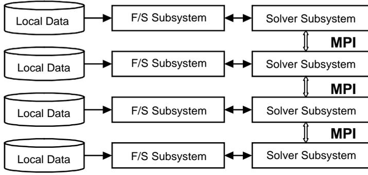
Figure 1: Global/Local Data Operation in GeoFEM
