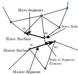
Figure 2: Node to segment model for complex faults.
