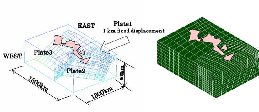
Figure 3: Analysis Model of Typical Faults Network at the 3 Plates End
