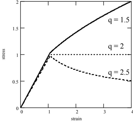
Fig.1 The one-dimensional stress and strain relation of the linear-elastic but heterogeneous-brittle model with different  $q$  values. It shows that the greater the mesoscopic strength scatter is, the softer the model becomes.
