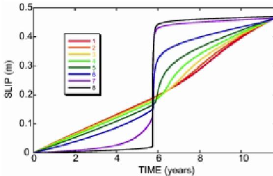
Figure 2: Simulated slip histories at 8 points on the fault during the entire cycle.
