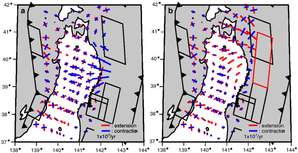
Figure 3: (a) Computed strain rate field in the Tohoku district during the period of 1897-1987. The barbed lines mark the plate boundaries. The rectangle regions correspond the horizontal projection of the faults for the interplate earthquakes, which occurred in analyzed period. (b) Including the effect of the virtual interplate earthquake. The red rectangle means the fault plane of the virtual earthquake.
